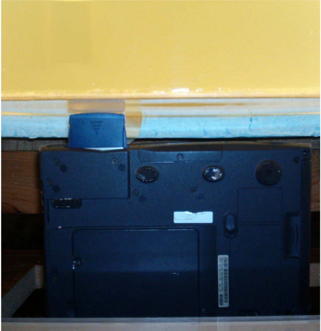
Fig. 3. Photograph of the Dell Model PP01L Host Computer at 90° with the edge of the Senao Model NL-5354 CB Plus Aries2 Cardbus Adapter pressed against the bottom of the planar phantom. This is Configuration 2 for SAR testing and represents the case of a bystander at a distance of 0 cm from the edge of the Cardbus Adapter.
