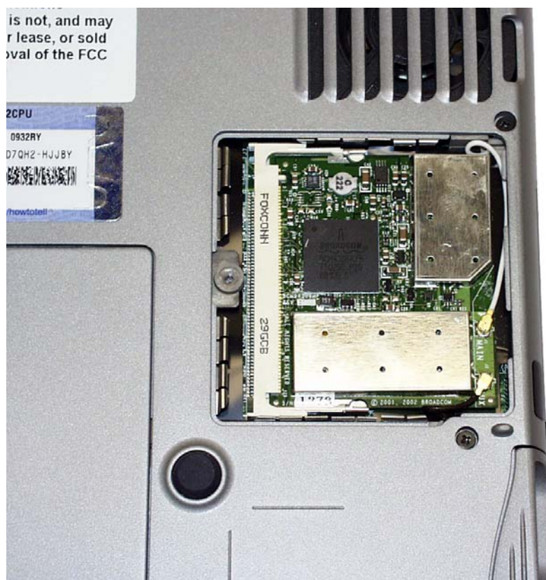
< D.U.T. installed in miniPCI slot >
