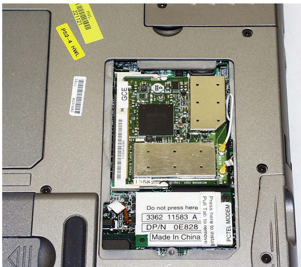
< D.U.T. installed in miniPCI slot >
