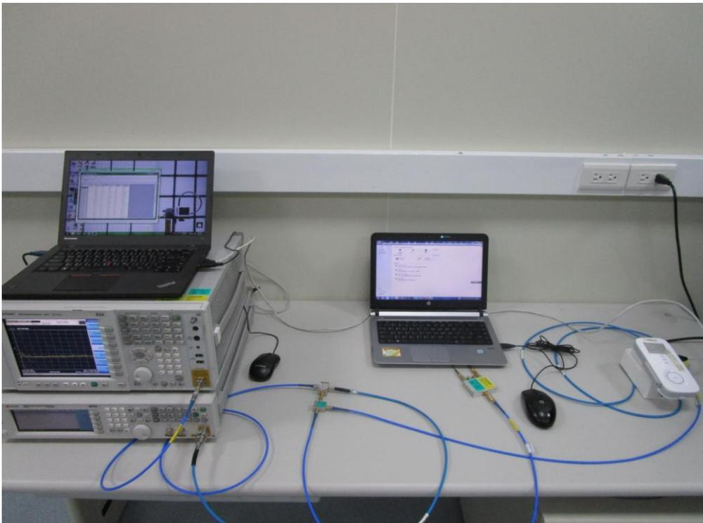
Description: DFS Radiated Measurement Test Setup
