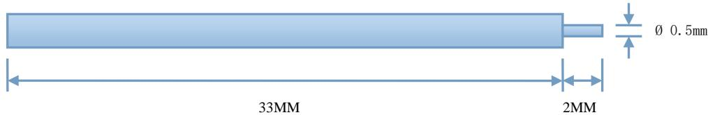
Antenna Type (天线类型) : Integrated antenna (一体化天线) ;
