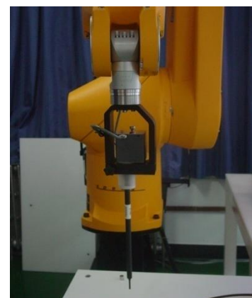
Picture C.2Near-field Probe
