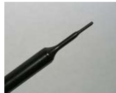
Picture C.2Near-field Probe
