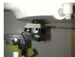
Figure 14.13 Body SAR Test Setup -- w/ Belt Clip --
