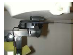
Figure 14.17 Body SAR Test Setup -- w/ Holster --
