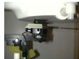
Figure 14.14 Body SAR Test Setup -- w/ Belt Clip --
