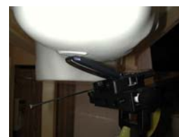
Figure 14.10 Right Head SAR Test Setup -- Ear / Tilt Position --
