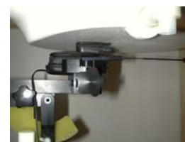
Figure 14.18 Body SAR Test Setup -- w/ Holster --
