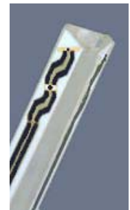
Figure 3.2 Probe Thick-Film Technique
