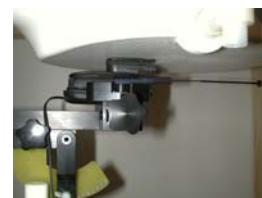
Figure 14.16 Body SAR Test Setup -- w/ Holster --
