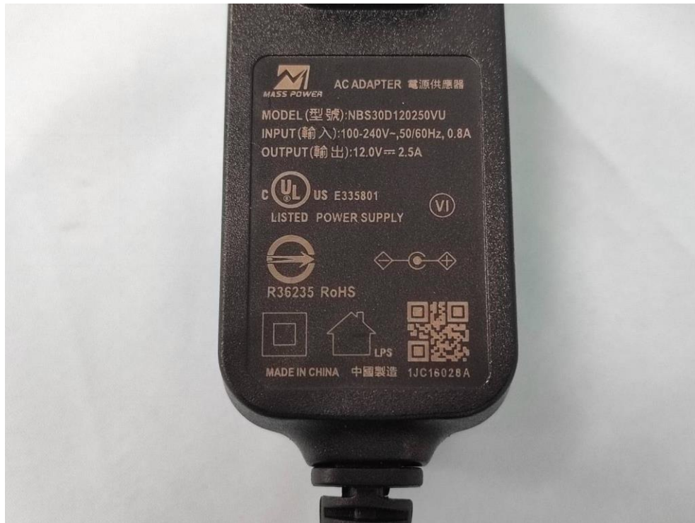
(13) Adapter(Brand: MASS POWER ,M/N: NBS30D120250VU)
