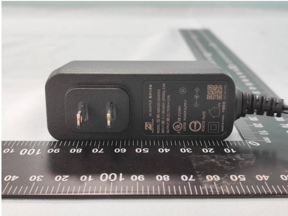
(10) Adapter(Brand: MASS POWER ,M/N: NBS30D120250VU)
