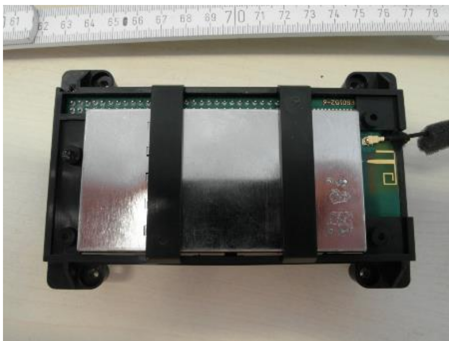
Photo 14: PCB 4 front side with aluminium shielding
