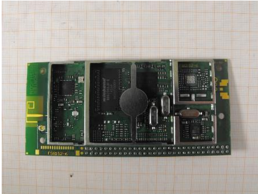
Photo 15: PCB 4 front side without aluminium shielding
