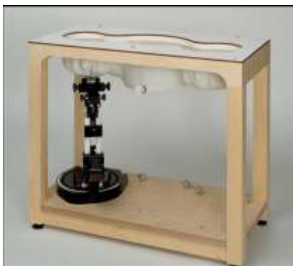
Picture C.10: SAM Twin Phantom
