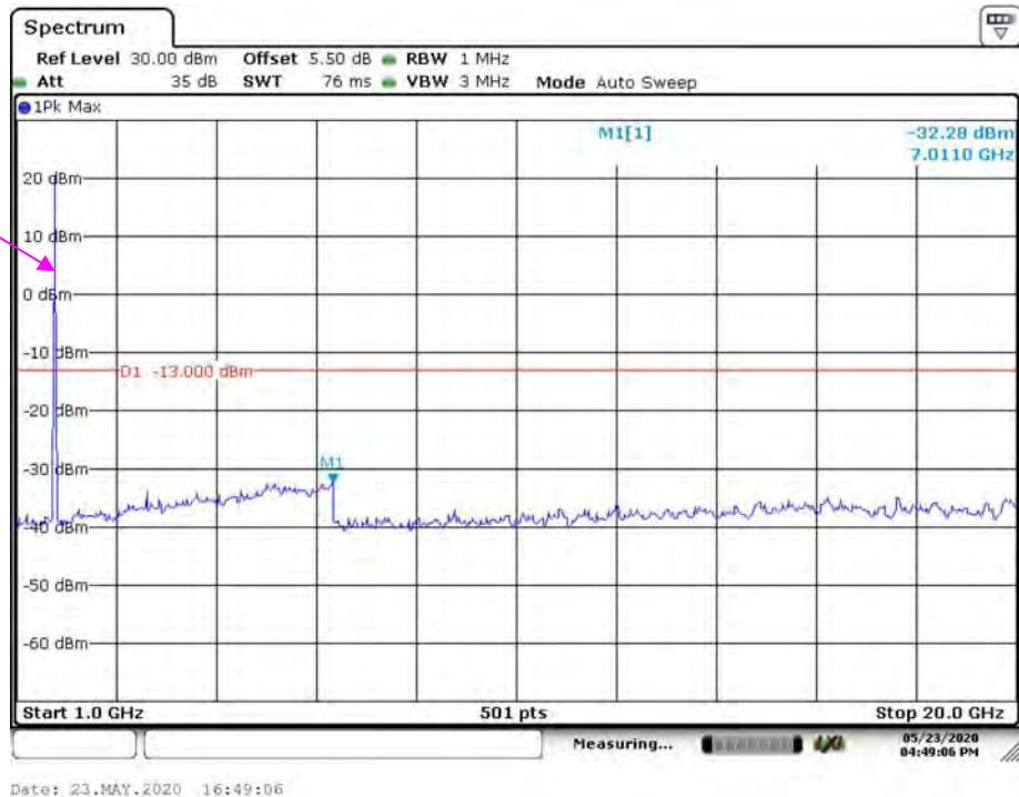
**LTE Band 66, 10 MHz QPSK Full RB Middle Channel**
