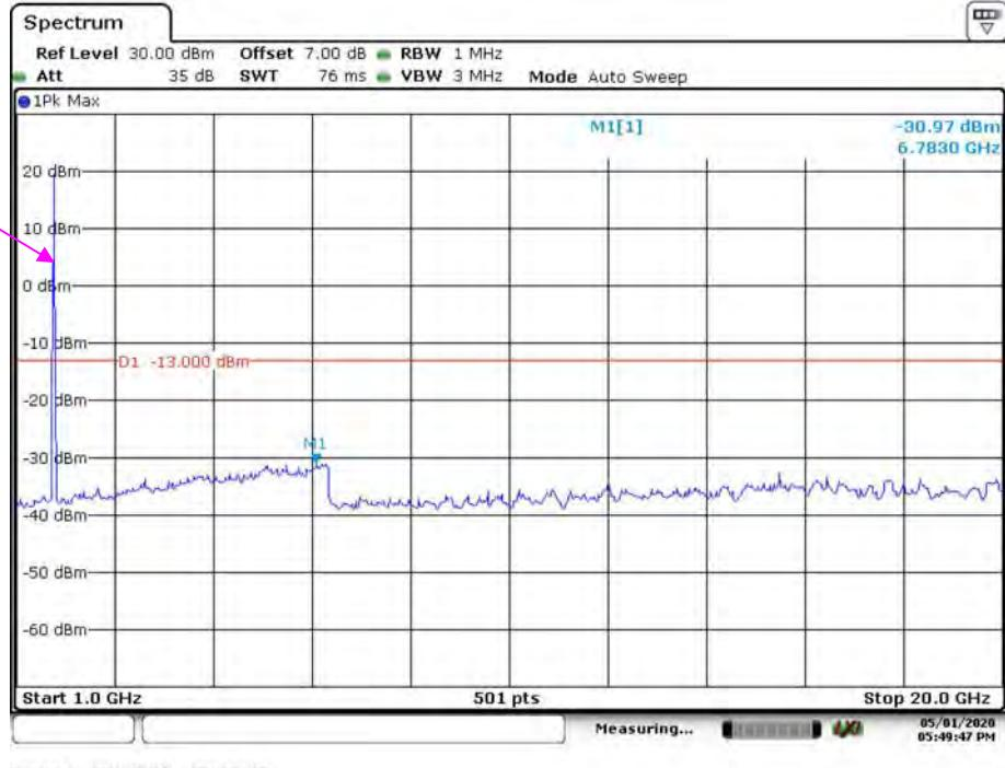
**LTE Band 4, 20 MHz QPSK Full RB Middle Channel**
