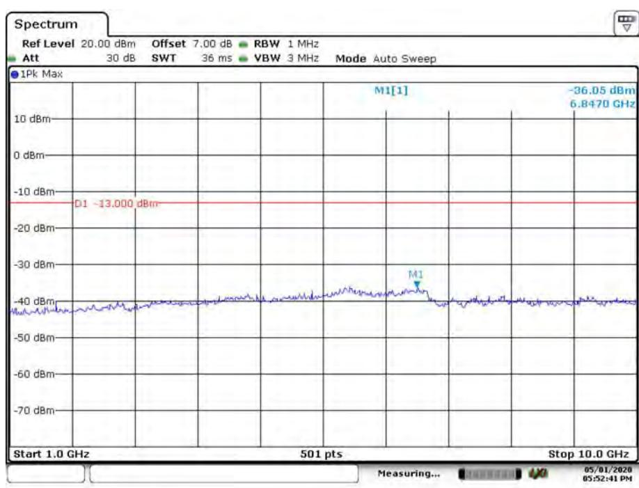
**LTE Band 5, 5 MHz QPSK Full RB Middle Channel**
