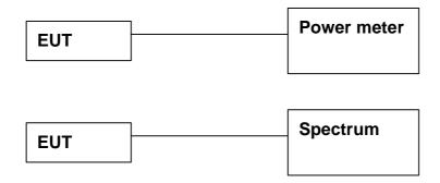
The EUT was connected to a spectrum through a 50 RF cable.
