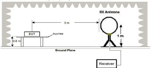
2. Radiated Emission Test-Up Frequency 30MHz~1GHz
