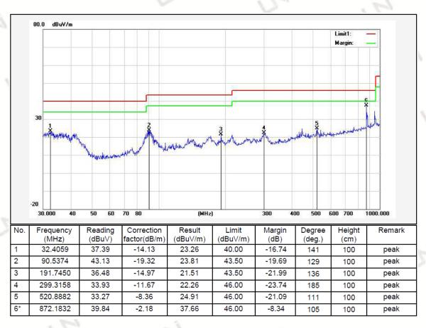
Remark: Result = Reading Level + Factor, Margin = Result - Limit Factor = Ant. Factor + Cable Loss - Pre-amplifier
