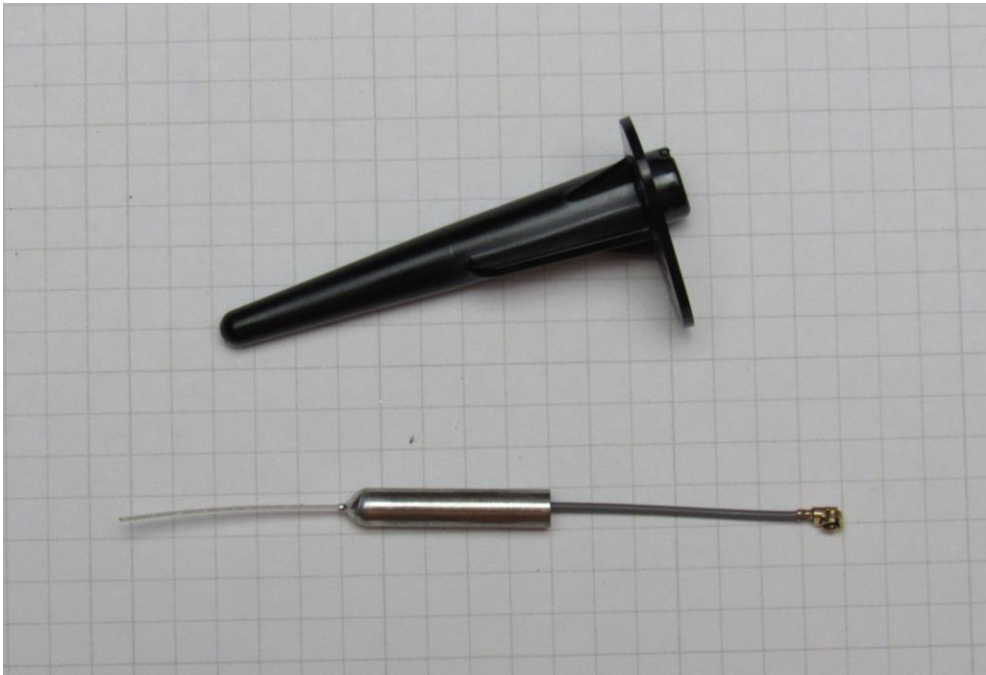
Antenna and “Antenna Holder” that is installed into “HUB Top”. Antenna slides into “Antenna Holder”. Grid pattern is 5mm.
