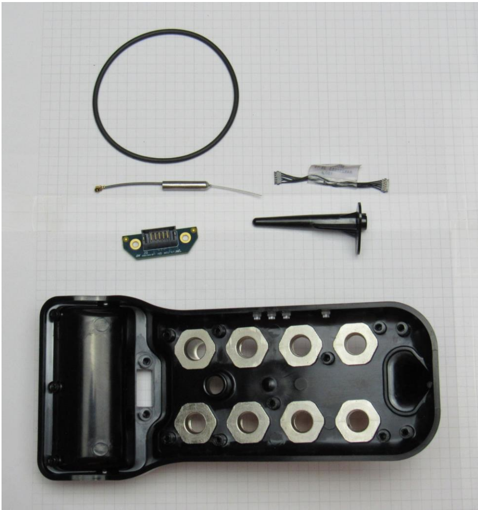
“HUB Top” and parts that are assembled into “HUB Top”. Grid pattern is 5mm.
