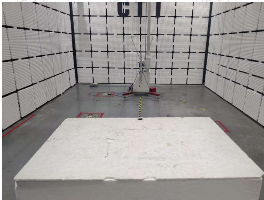
Radiated spurious emission Test Setup-1(Below 1GHz)
