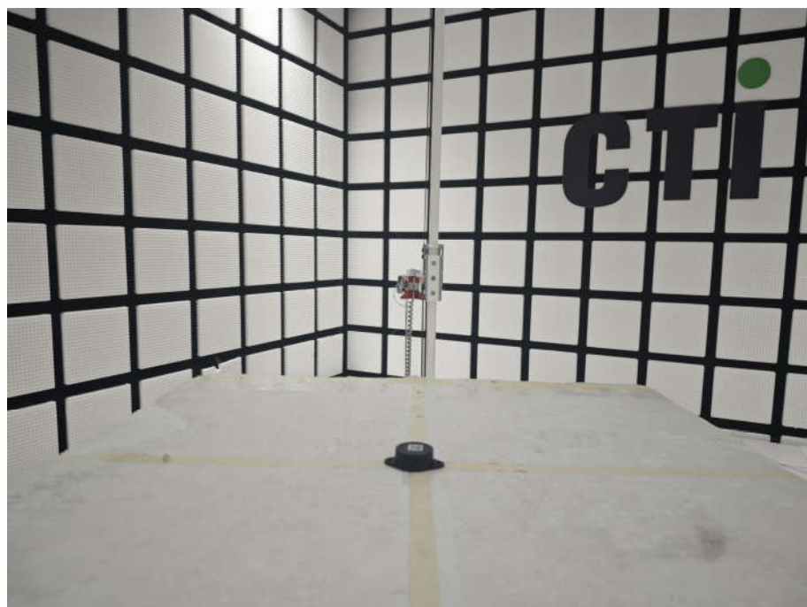
Radiated spurious emission Test Setup-3(Above 1GHz)
