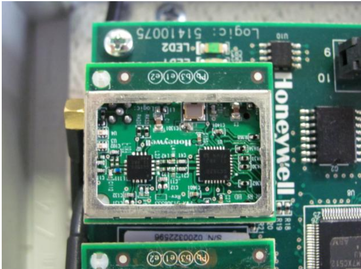
Figure 2. Radio 1 with Shielding Removed
