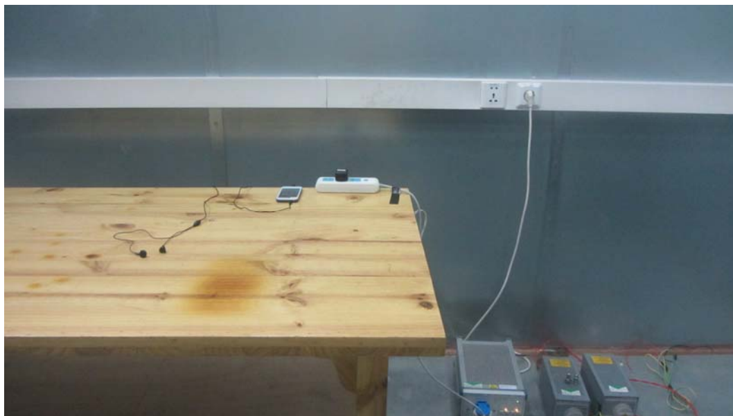
Picture 3 Conducted Emission Test Setup
