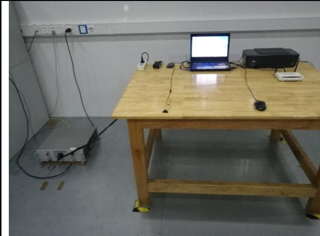
Conducted Emissions Test Setup – Front View
