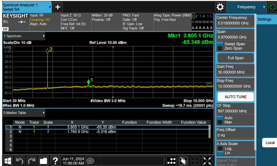
Sub6 n66_15 M_Conducted Spurious(30 M-10 G)_High_BPSK_1RB
