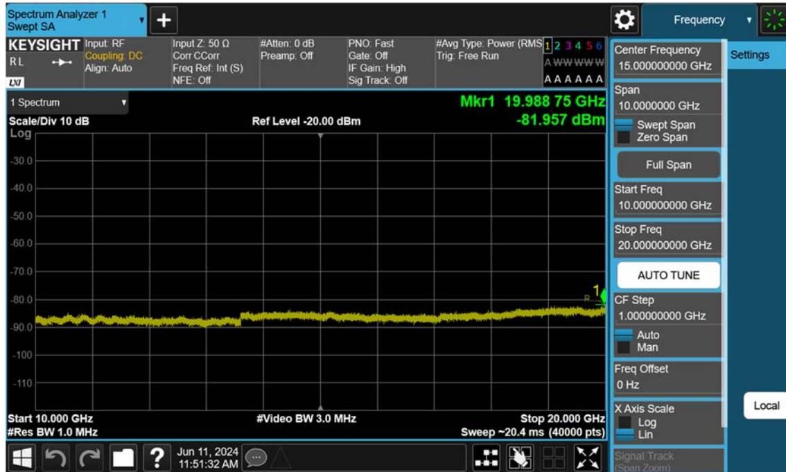
Sub6 n66_15 M_Conducted Spurious(Above10 G)_Low_BPSK_1RB
