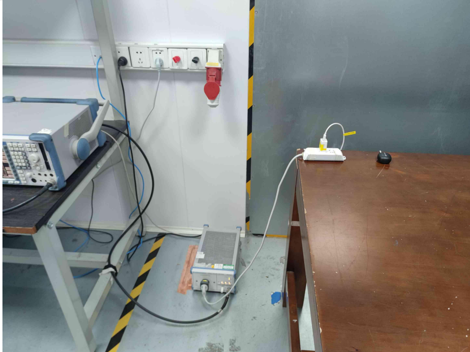
Conducted emissions at AC power line (150kHz-30MHz)
