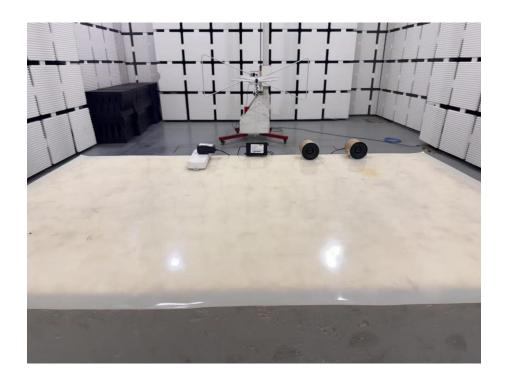
**Set-up for Radiated Spurious Emission, Above 1GHz**
