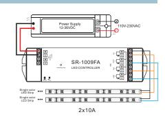
2)Receiver Connection Diagram for Multiple Units
