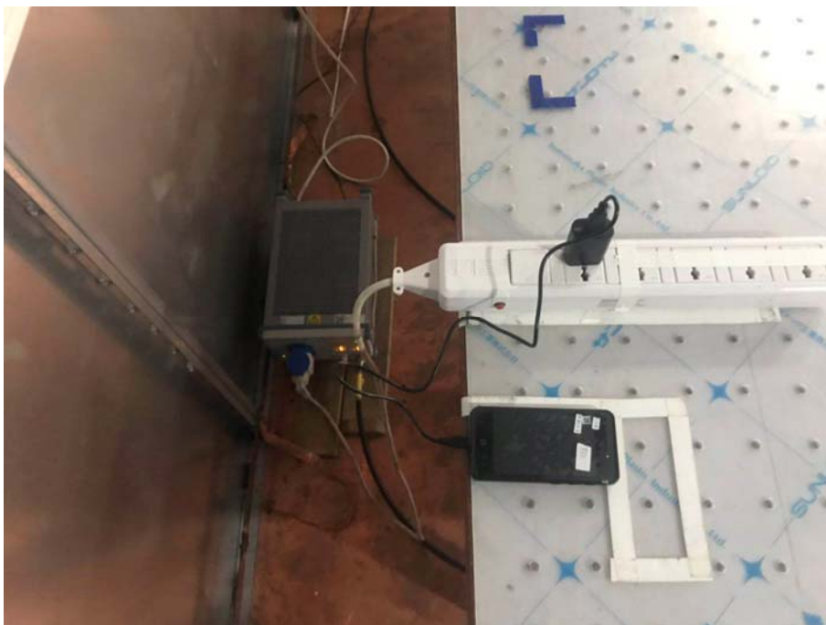
Conducted Emissions Test Setup (with charger)
