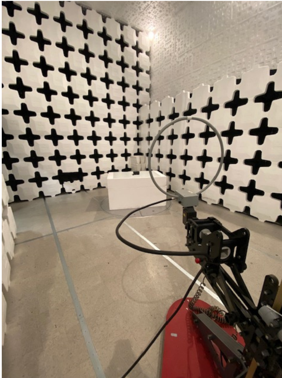
Figure 7. Radiated Emissions Test Setup, 9 kHz to 30 MHz (Normal Operation), Outdoor Unit
