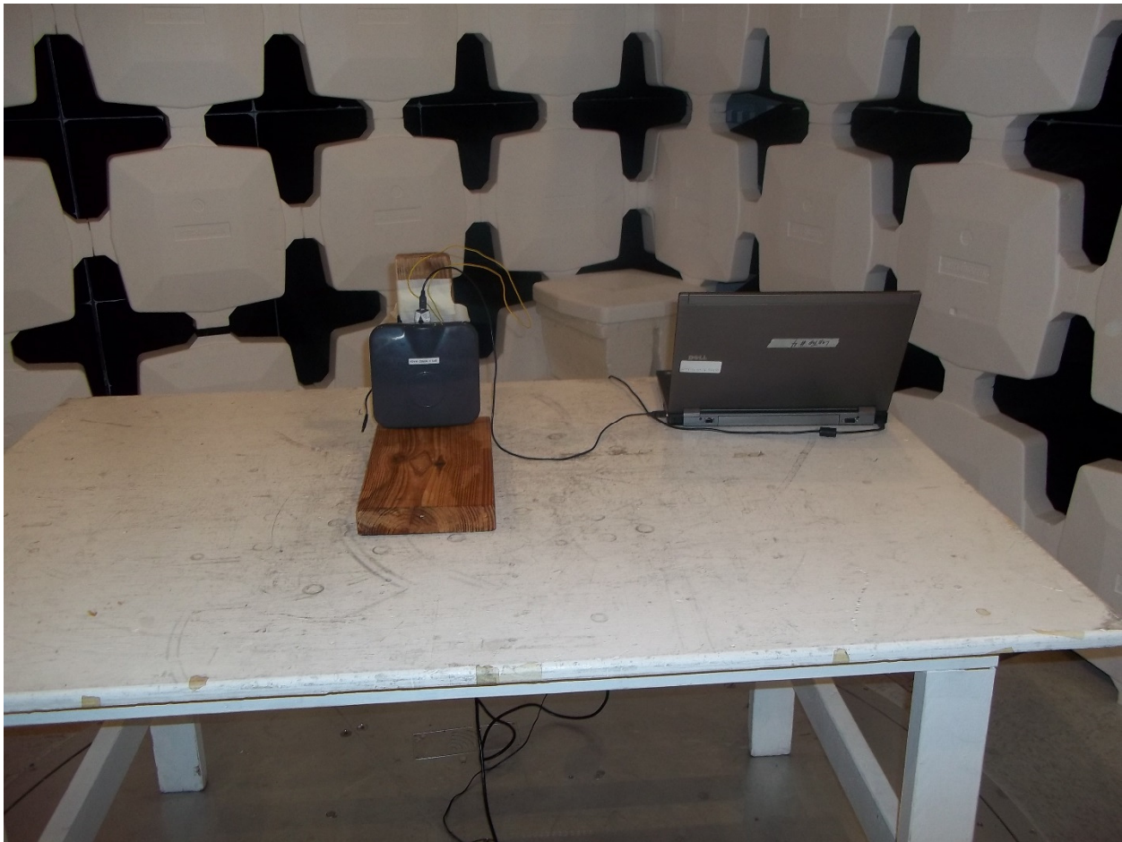
Figure 1. Radiated Emissions Test Setup, Close-Up, Indoor Unit
