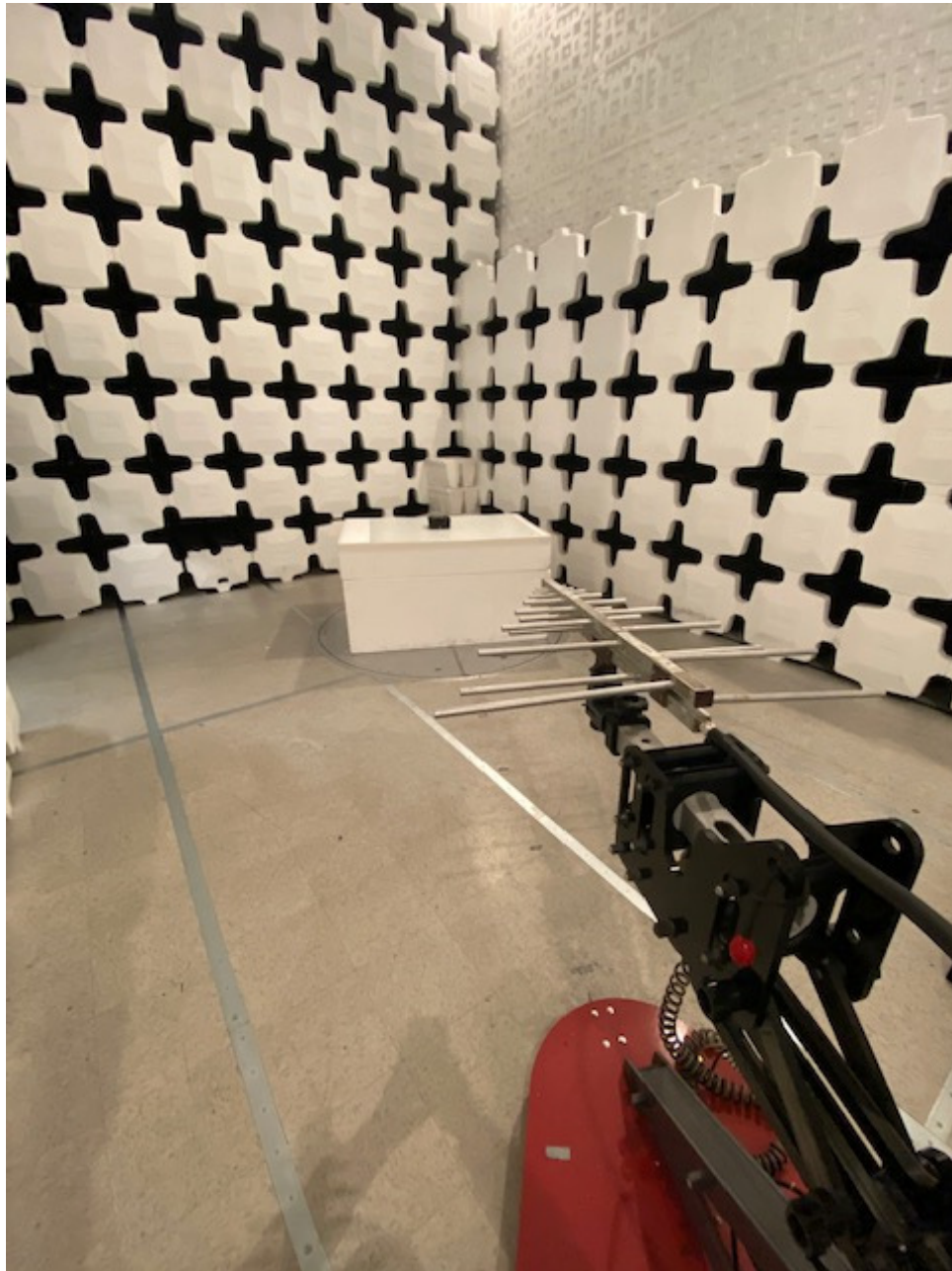
Figure 9. Radiated Emissions Test Setup, 200 MHz to 1 GHz (Radio Test with EUT in worst case position), Outdoor Unit
