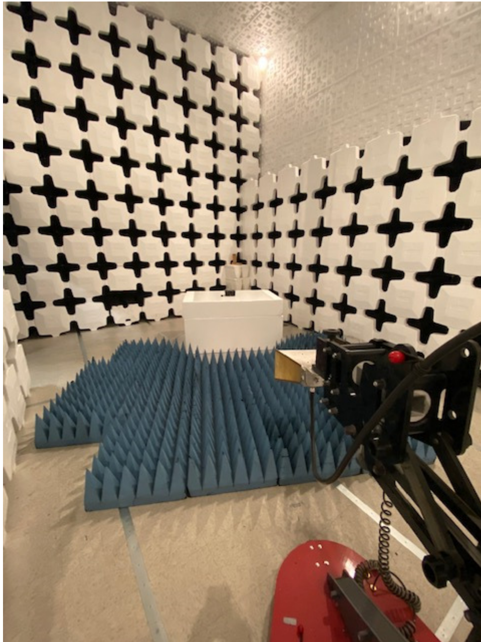
Figure 10. Radiated Emissions Test Setup, Above 1 GHz (Radio Test with EUT in worst case position), Outdoor Unit
