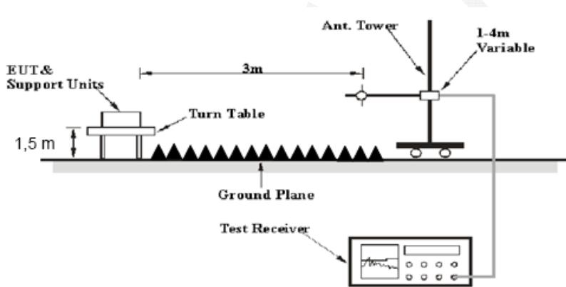
The radiated emission tests were performed in the 3 meters test site, using the setup accordance with the ANSI C63.10-2013. The specification used was the FCC 15.209, and FCC 15.247 limits.
