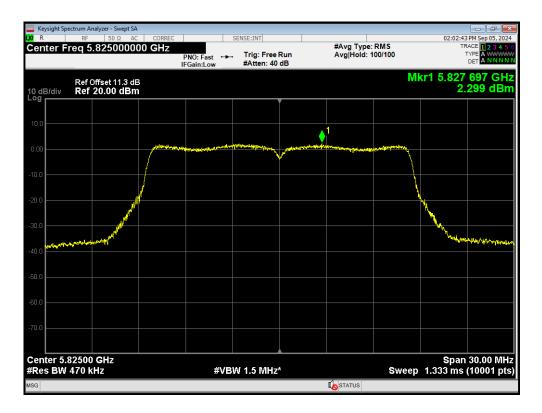
PSD 802.11ac(VHT20) 5745MHz
