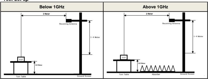
These measurements were performed at 3 m test site. The equipment under test is placed on a non-conductive table 0.8 m or 1.5 m above a turntable which is flush with the ground plane and 3 meters from the receive antenna. For measurements above 1 GHz absorbers are placed on the floor between the turn table and the antenna mast in such a way so as to maximize the reduction of reflections. For measurements below 1 GHz, the absorbers are removed.
