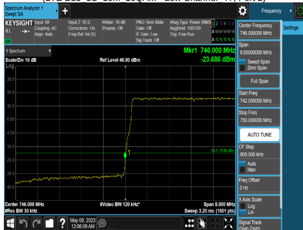
Plot 8-413. Band Edge Emission Summary Data Plot (LTE B13 2C 5M+5M QPSK - Low Channel 4T, Port 1)
