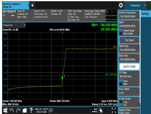
Plot 8-421. Band Edge Emission Summary Data Plot (Multi-Band_LTE B13_2C_5M+5M+DSS B(n)5_1C_10M+NR n5_1C_10M+LTE B5_1C_5M_QPSK - Low Channel_4T, Port 3)
