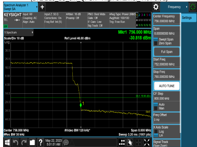
Plot 8-412. Band Edge Emission Summary Data Plot (LTE B13 1C 10M QPSK - High Channel 4T, Port 2)
