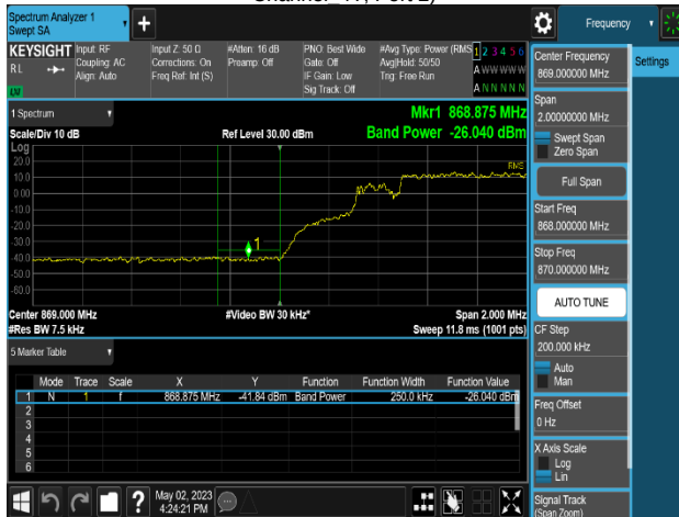
Plot 8-399. Band Edge Emission Summary Data Plot (MSR 2C_DSS B(n)5_1C_10M+NR n5_1C_15M_16QAM - Low Channel 4T, Port 1)
