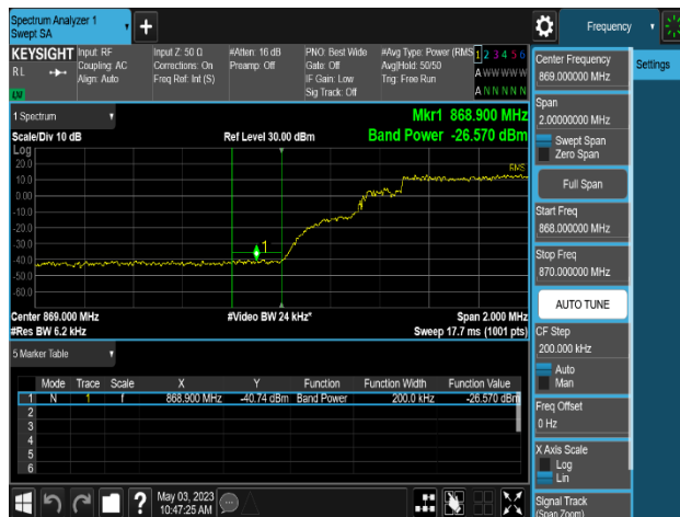
Plot 8-403. Band Edge Emission Summary Data Plot (MSR 3C_DSS B(n)5_1C_10M+NR n5_1C_5M+LTE B5_1C_5M_16QAM - Low Channel 4T, Port 2)
