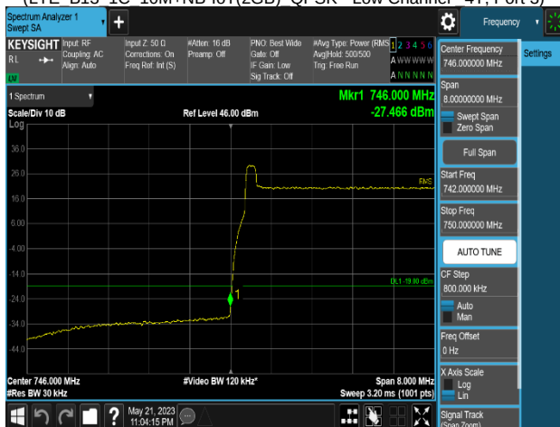
Plot 8-419. Band Edge Emission Summary Data Plot (Multi-Band_LTE B13_1C_10M+B5_1C_10M_QPSK - Low Channel 4T, Port 3)
