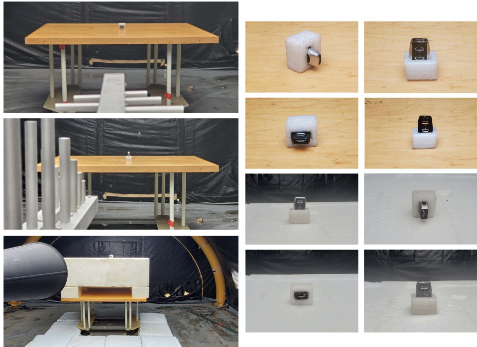
Figure 4: Radiated Emissions Test Setup Photograph(s).
