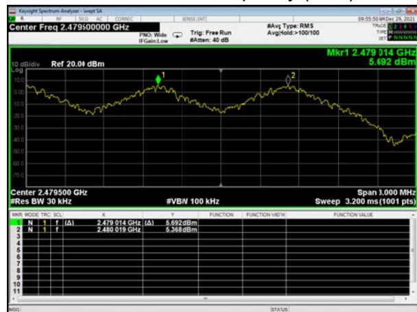
BT DH5 CH78, Carrier frequency (MHz): 2480
