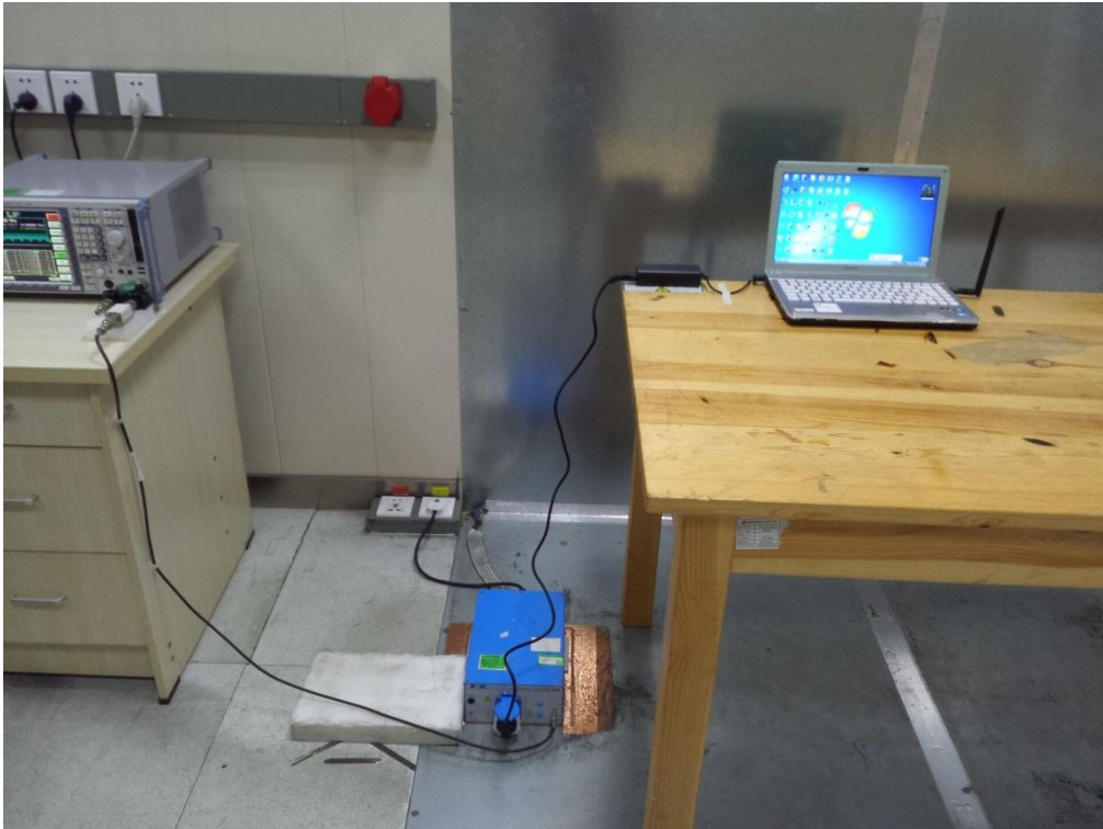
RADIATE EMISSION TEST SETUP ABOVE 1GHz
