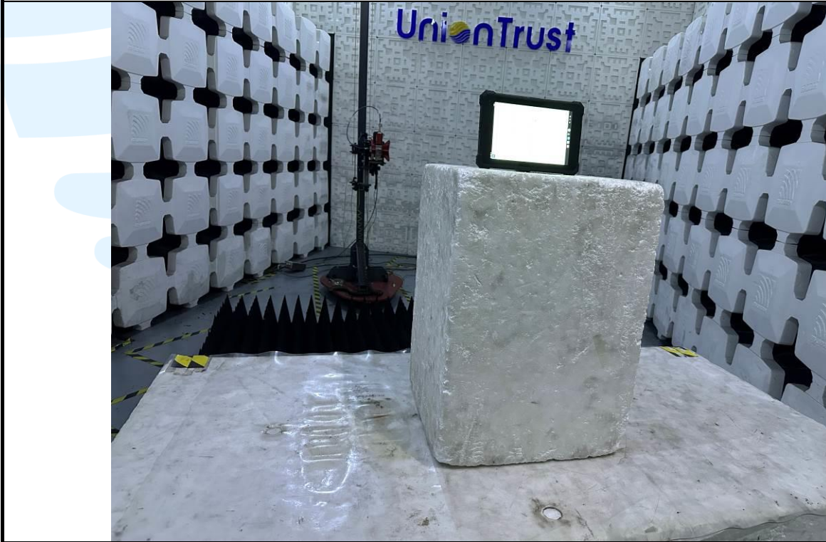
Radiated emission Test Setup (Above 1 GHz)
