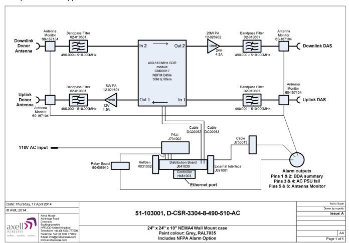
Figure 1. UHF D-CSR3304 for Type approval – Part number 51-103001.
