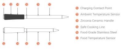
Note: Only the long black probe can detect ambient temperatures, the white probe cannot.
