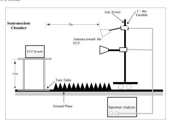
The radiated emissions were performed in the 3 meters distance, using the setup accordance with the ANSI C63.10-2013. The specification used was the FCC 15.209, FCC 15.247 limits & RSS-247, RSS-Gen limits.
