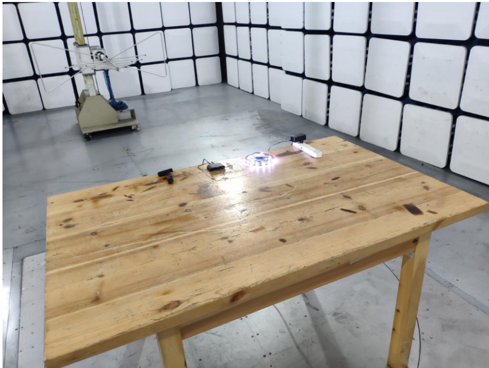
Photo of Radiation Emission Test
