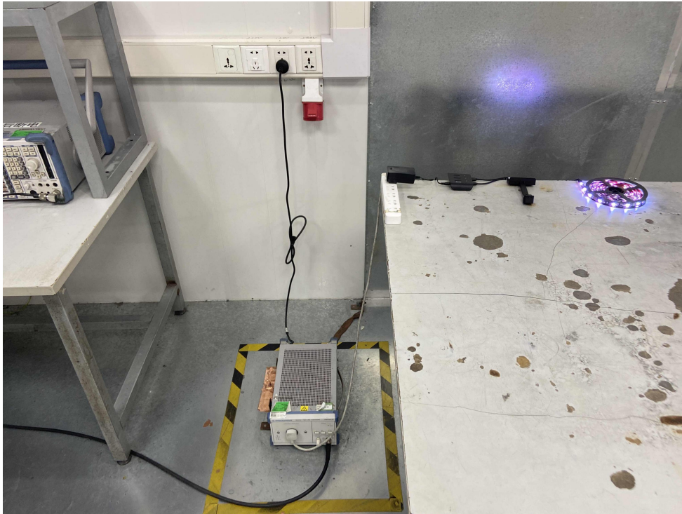
FCC ID: 2AQA6-H6199 Photo of Power Line Conducted Emission Test
