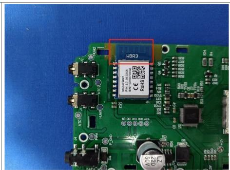
The antenna is PCB antenna. The best case gain of the antenna is 2.54 dBi. wifi and Bluetooth cannot be transmitted at the same time
