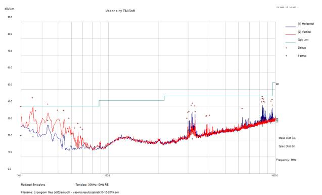
Turntable Corrected Antenna Antenna **Frequency** Limit Margin Amplitude Height **Polarity Azimuth Comment**  $(dB\mu V/m)$ (dB) (MHz)  $(dB\mu V/m)$ (H/V)(cm) (degrees) 35.54875 22.09 280 V 304 -17.91 40 QP V 225 43.52075 31.89 138 40 -8.11 OP V 30 22.72 199 162 40 -17.28 QP 836.377 33.61 107 Η 167 46 -12.39 QP 840.20225 28.42 129 Η 117 46 -17.58 QP 319.6815 20.9 125 Η 272 46 -25.1 QP
