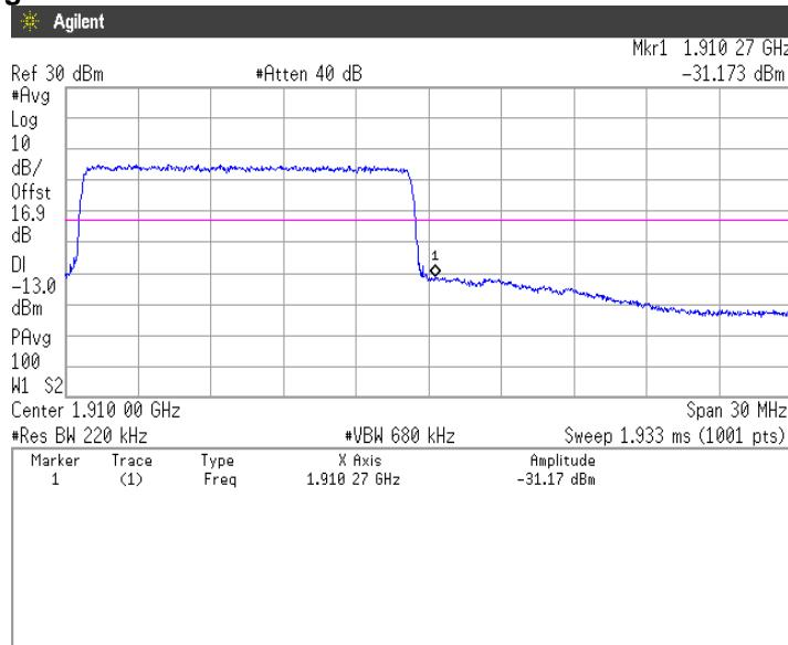
**16QAM, BW 20MHz, RB1-0****Channel: Low**
