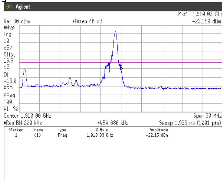
**QPSK, BW 15MHz, RB75-0****Channel: Low**
