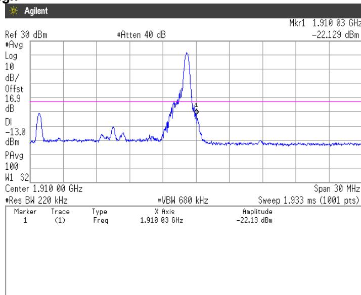
**16QAM, BW 15MHz, RB75-0****Channel: Low**
