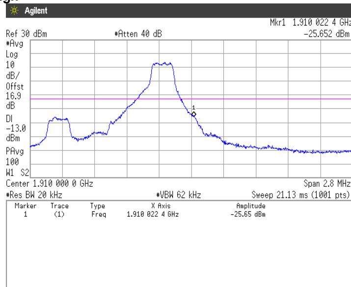
**16QAM, BW 1.4MHz, RB6-0****Channel: Low**
