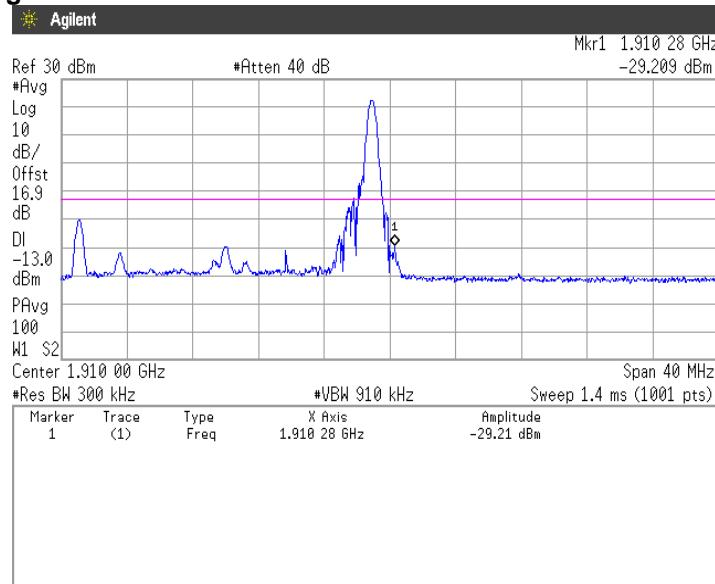
**QPSK, BW 20MHz, RB100-0****Channel: Low**
