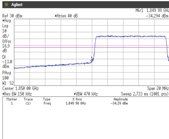
**16QAM, BW 10MHz, RB50-0****Channel: High**
