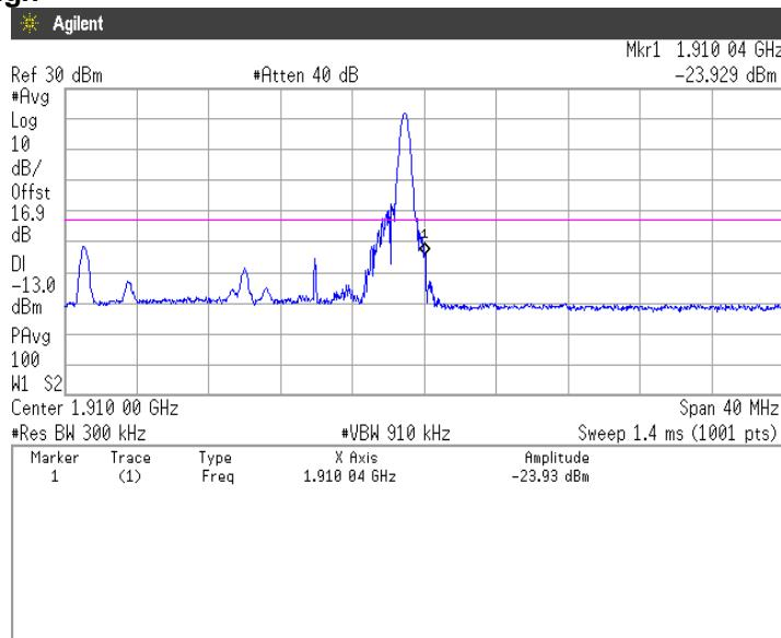
**16QAM, BW 20MHz, RB100-0****Channel: Low**
