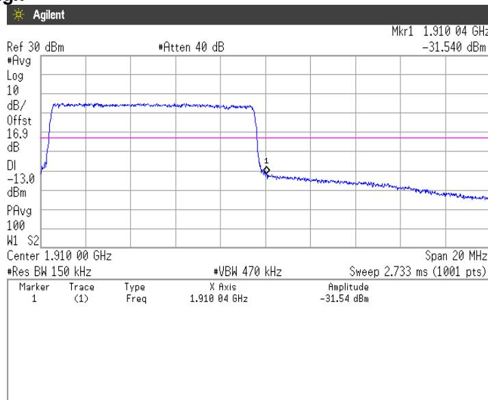
**16QAM, BW 15MHz, RB1-0****Channel: Low**
