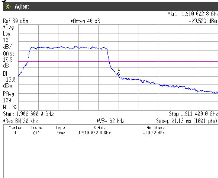
**64QAM, BW 3MHz, RB1-0****Channel: Low**
