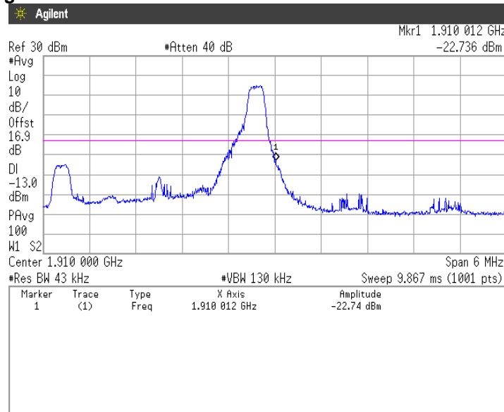
**64QAM, BW 3MHz, RB15-0****Channel: Low**
