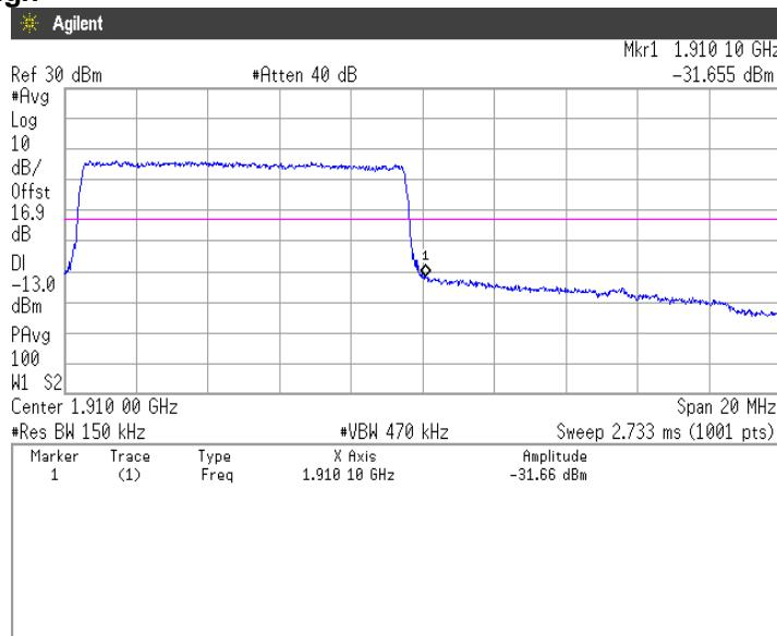
**QPSK, BW 15MHz, RB1-0****Channel: Low**
