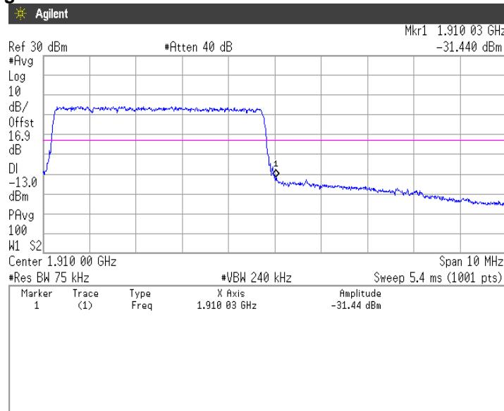
**64QAM, BW 10MHz, RB1-0****Channel: Low**
