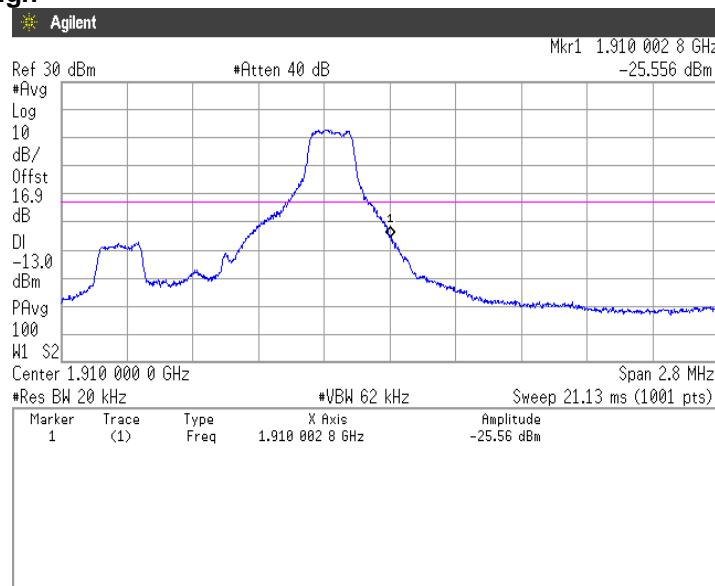
**64QAM, BW 1.4MHz, RB6-0****Channel: Low**
