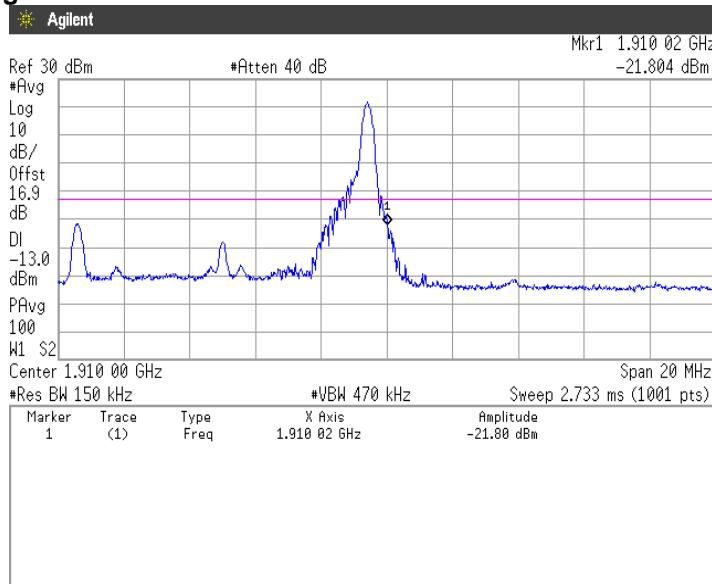
**16QAM, BW 10MHz, RB50-0****Channel: Low**
