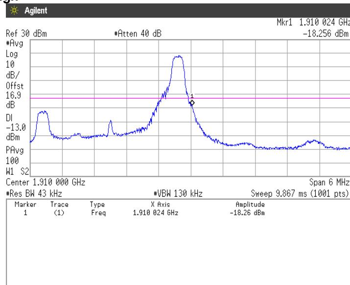
**QPSK, BW 3MHz, RB15-0****Channel: Low**
