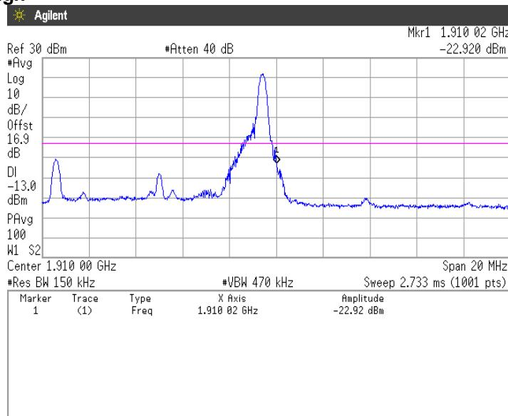
**QPSK, BW 10MHz, RB50-0****Channel: Low**
