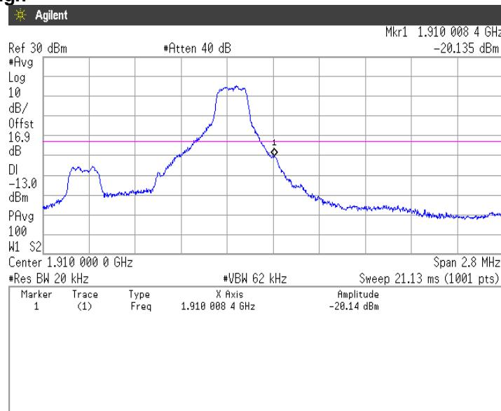
**QPSK, BW 1.4MHz, RB6-0****Channel: Low**
