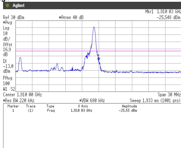
**64QAM, BW 15MHz, RB75-0****Channel: Low**
