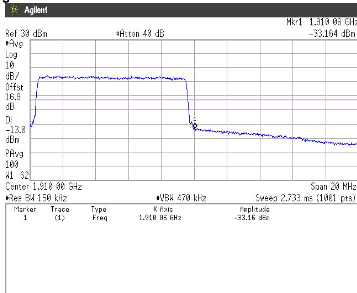
**64QAM, BW 15MHz, RB1-0****Channel: Low**
