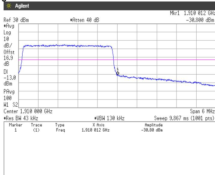
**16QAM, BW 5MHz, RB1-0****Channel: Low**
