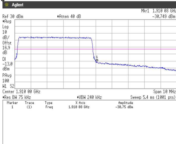
**16QAM, BW 10MHz, RB1-0****Channel: Low**
