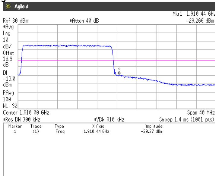
**16QAM, BW 1.4MHz, RB1-0****Channel: Low**
