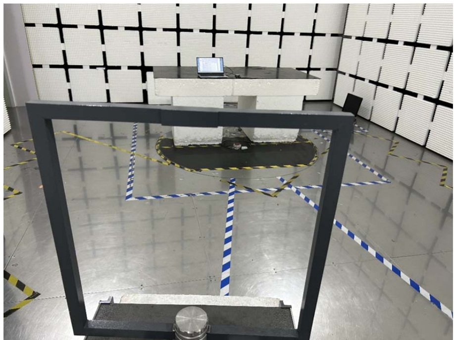
Radiation Emission Test Setup (Below 30MHz)
