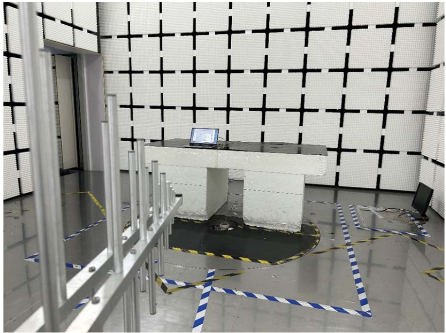
Radiation Emission Test Setup (30MHz to 1GHz)
