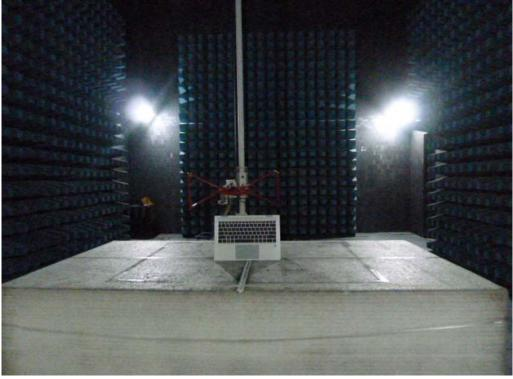
Radiated Emission Set up Photos (Above 1GHz)
