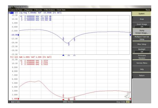
This plots shows that the VSWR response of the antennas tested were within the specified range which is <2:1.
