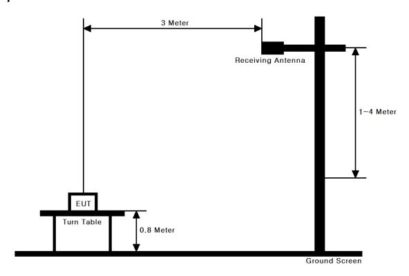
These measurements were performed at 3&10m test site. The equipment under test is placed on a non-conductive turntable 0.8-meters above the ground plane and 3-meters from the receive antenna.
