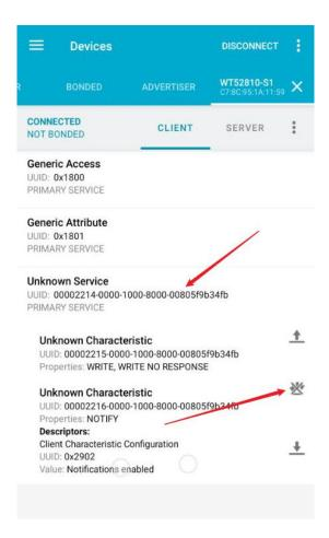
Then, the NOTIFY channel can receive the serial port data, or send data to the serial port through the WRITE, WRITE NO RESPONSE channel.
