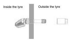
1.4 Place nut<sup>®</sup> on the valve stem, and tighten with 5 Nm (44 inch pounds) torque.
