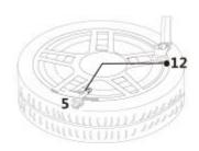
1.7 Apply soapsuds on the valve tip. If no leakage is found, put on the valve cap<sup>6</sup>. If unsuccessful, try again.
