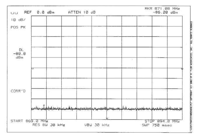
POWER: MODULATION: LOW ANY TX SPURS IN RX CRITICAL BAND
