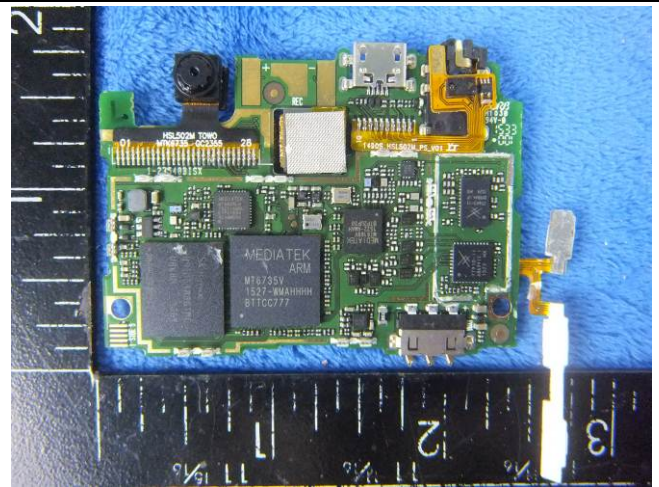
Mainboard without Shielding - Rear View
