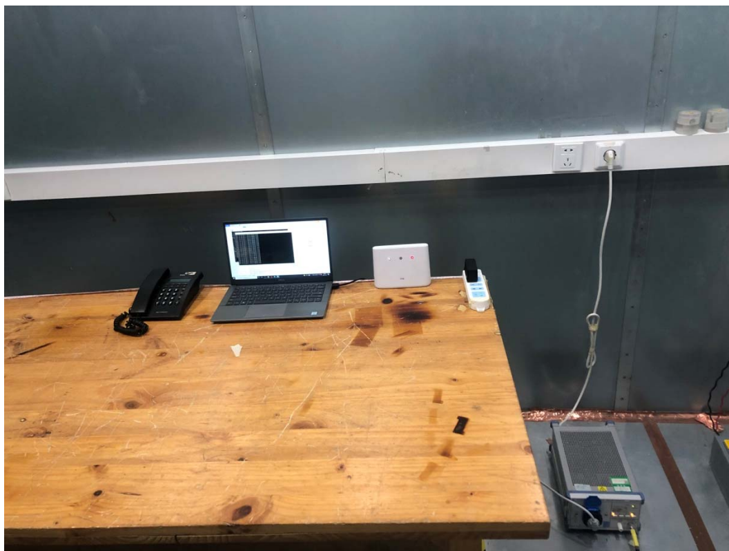
Picture 2: Conducted Emissions Test Setup
