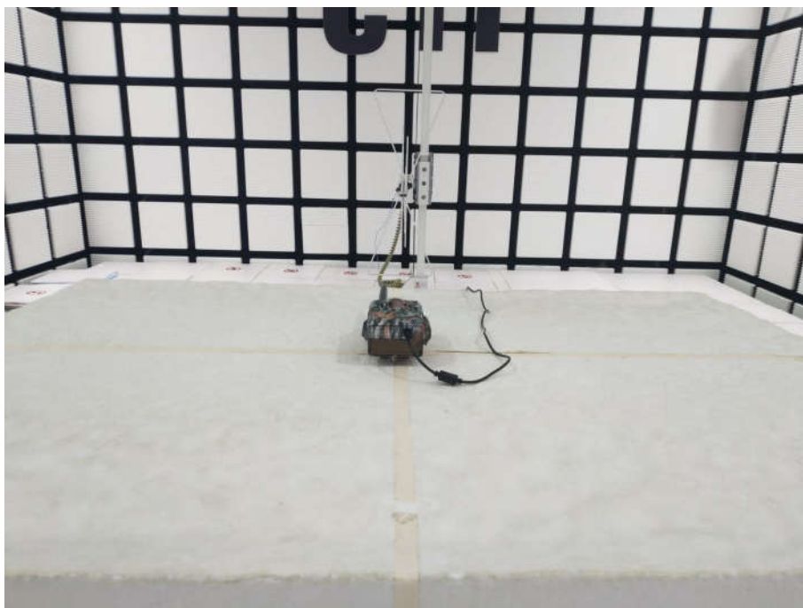
Radiated spurious emission Test Setup-1(Below 1GHz)
