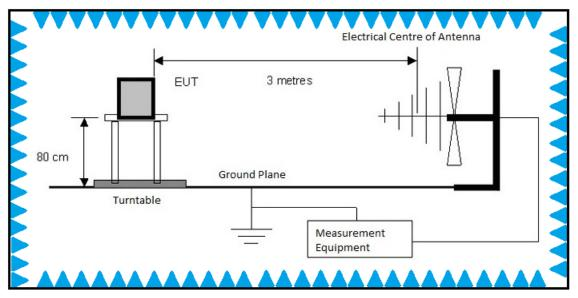
Test setup diagram for Radiated Spurious Emissions testing (above 1GHz):
