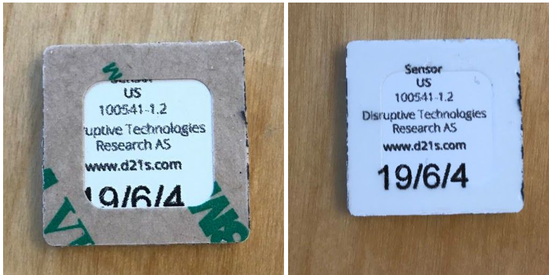
Figure 2: Images of back side of PN 100541 Sensor US, DT white unprinted Sensor (Node0), single, with transparent backing tape. In the image to the right, the protection foil of the transparent backing tape has been removed. The transparent backing tape is present to enable easy assembly onto e.g. a wall.
